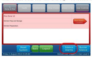
2) The cause of the fire condition can be determined through the touch screen display, it will show the device(s) that triggered the system into alarm. Note: Smoke detectors will not reset until they are clear of smoke, heat detectors will not reset until the temperature has reduced below the trigger threshold. Callpoints can be reset by glass replacement, removal of the test key (if it was a test) or resetting the non-frangible element.
